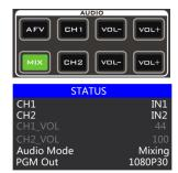
2. The mixing assigned channels are IN1、IN2、IN3、IN4、PHONE\_IN、MIC\_IN1、MIC\_IN2. Under the mixing assignment mode, there are two more audio embedding functions; PHONE\_IN means 3.5mm stereo audio interface, MIC\_IN means 3.5mm microphone audio interface; PGM live output can mix two audio channels at any time, and the volume of the two audio channels can also be adjusted separately.
