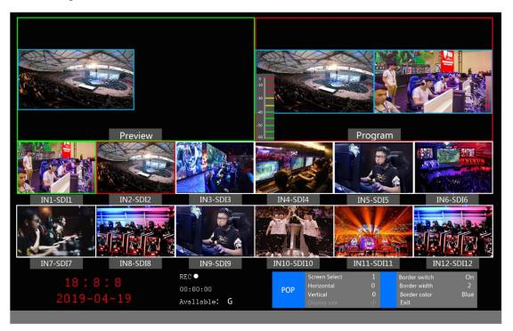
At this time, the information on the LCD screen will be switched to the POP picture-out-picture setting, and the knob can be set as required. As shown below
