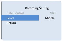
The level can be set in the recording settings, and can be set with low, middle, high and super high.
