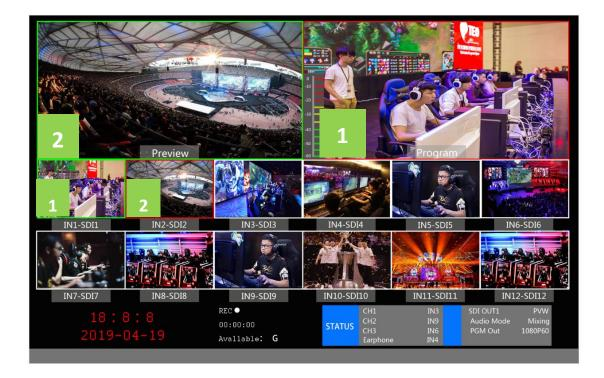
Then press the AUTO, CUT, or manually push the fader on the control panel to switch.
