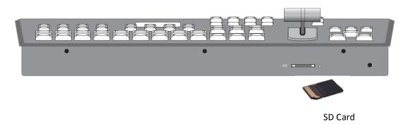
You can use the SD card to record video. After inserting the SD card normally, press the REC button to record the PGM output video. To pause, you can click the PAUSE button.
