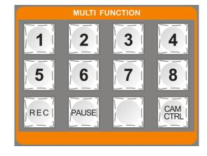
Recording button, after the SD card is normally inserted, the red light is displayed after pressing REC
