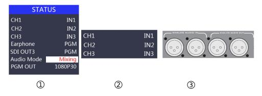
2. Operate the mixer control area, press the SRC1 button to enter the first audio channel to select IN1, IN2, IN3, IN4, IN5, IN6, IN7、IN8、IN9 、IN10、IN11、IN12、XLR\_IN. The corresponding menu status bar will change according to your choice in real time.
