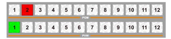
Press the selection in the PGM area as shown above, and the button will turn red (live). Pressing PVW will display green (pre-supervised).
