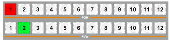
If you want to display the source of the SDI1 interface on the PVW, the source of the SDI2 interface is displayed on the PGM press the 1 button directly in the PVW area, and press PGM to press 2. As shown above
