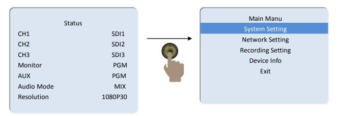
Rotate the knob under the status bar to set the auxiliary output, audio mode, and output resolution;
