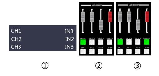
3. Operate the mixer control area, press the SRC2 button to enter the second audio channel to select IN1, IN2, IN3, IN4, IN5, IN6, IN7、IN8、IN9、IN10、IN11、IN12、XLR\_IN. The corresponding menu status bar will change according to your choice in real time.
