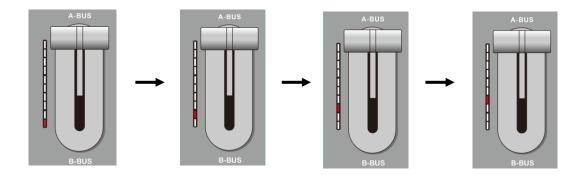
At this time, push the T-bar back and forth until the indication is normal. (All lights up or all lights down) as shown below.
