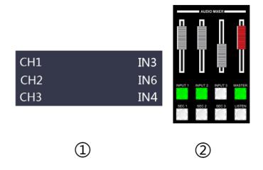
4. Operate the console control area and press the SRC3 button to enter the third audio channel and select IN1、IN2、IN3、IN4、IN5、IN6、IN7、IN8、IN9、IN10、IN11、IN12、XLR\_IN,The corresponding menu status bar will be based on your selection in real time. Change (as shown in Figure 1)
